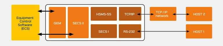
The software includes SECS-I/HSMS, SECS-II communication layers as well as GEM protocol communication capacity along with a C# API to gain an object-oriented access to the equipment communication interface. Full equipment integration can be reached through the Agileo Automation SECS/GEM driver no matter what level of communication protocol or communication line required by the equipment.
